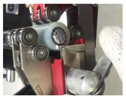
Rotate switch B to stretch the blade out, adjust the blade to make it in between the main insulation layer and the inner semi-con layer.
