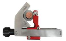
1) Rotate switch A, open the clamp to grip the cable main insulation layer, tighten the clamp up to grip the cable firmly.
