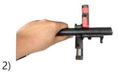
Adjust the blade depth switch C to the required spot and then rotate stripper B, leave a 360° cutting mark on the cable outer semi-con layer.
