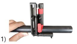
Grip the cable outer semi-con layer with locator A and stripper B according to the outer semi-con layer stripping length.
