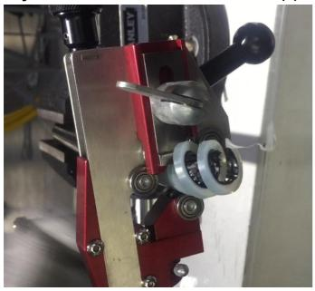
8. CST240 Insulation Chamfer Tool
