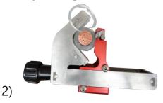
Rotate the tool and then the blade will form a chamfer in main insulation end.
