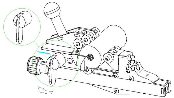
3. Adjust the knob C for the in feed position, clockwise rotate the tool, and slightly push to the direction of the cable, begin stripping work. After the stripping is completed, feed the knob C back to the flat cut, as shown in Figure below.
