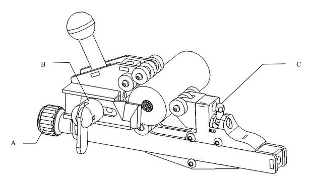
2. Rotate Loosen the handle B, manually remove the cutting blade, so that the blade reaches the main insulation and between the semi-conductive layer (careful not to scratch the cable core) and then
