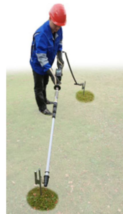
Check earth by second earth spike
