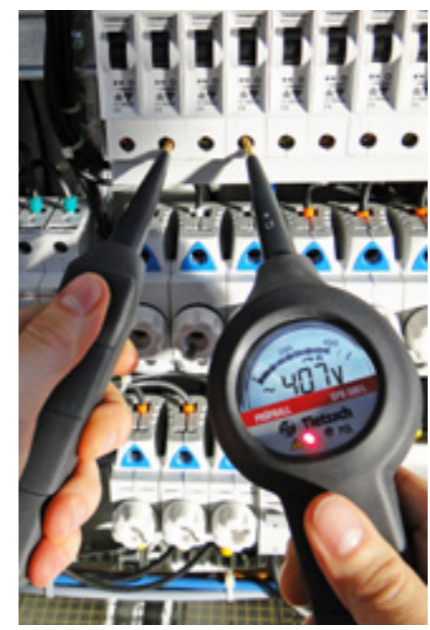
Direct voltage indication without pressed buttons
