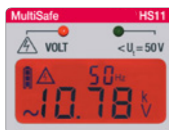
Colour change of the display at voltage
