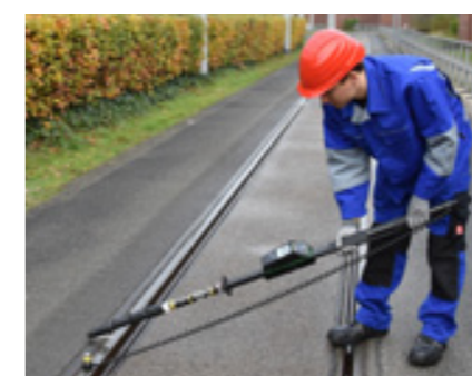
Complete self-test of device function and contact with the rail within seconds
