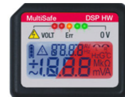
Display with bright LEDs and two-color LCD
