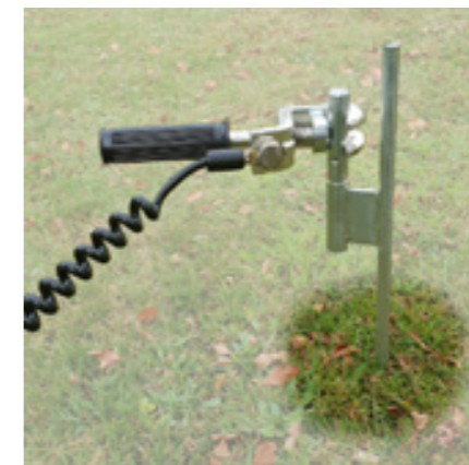
Earth connection with earthing spike and universal clamp
