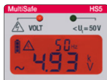
Colour change of the display at voltage
