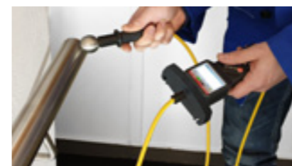
Testing of stair rails that protrude into the water
