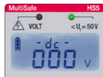
Indication of absence of voltage
