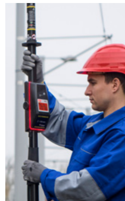
Direct indication of voltage on the LCD and warning by LED and acoustic signal.
