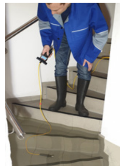
The ball electrode probes voltage in the water from a safe distance
