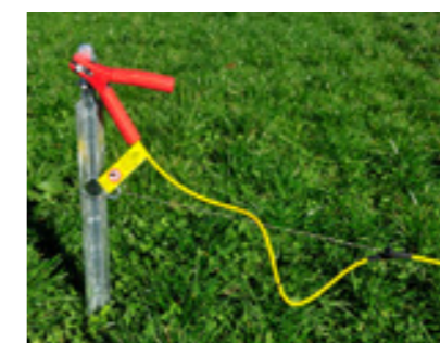
Earth connection, e.g. with earthing spike through clamp with strain relief
