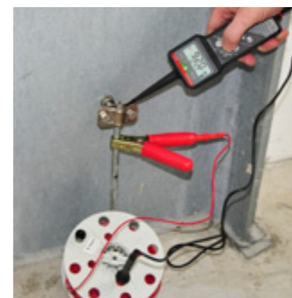
Quick compensation of the measuring line
